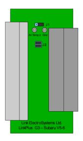
Jumper J2 sets the Immobiliser option. For vehicles without an immobiliser system, set the jumpers as shown to the left ('No Immobiliser' position). If the vehicle has an immobiliser, fit the jumpers in the 'Immobiliser' position.
